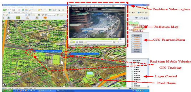
Fig. 6. The Screen Copy of Real-time Monitoring of Mobile Vehicles and Video Capture of a Road Cross
